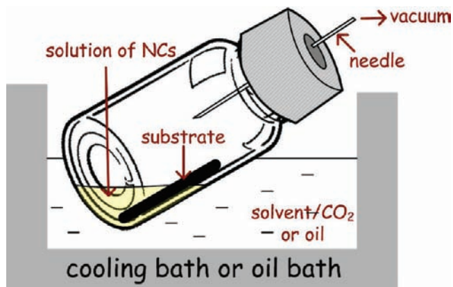
Figure 1. Setup used for studies of self-assembly of different nanocrystals into single-component and binary superlattices at various temperatures.
